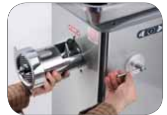
2. Sbocco bocca TC 32/ICE Head locking TC 32 / ICE
