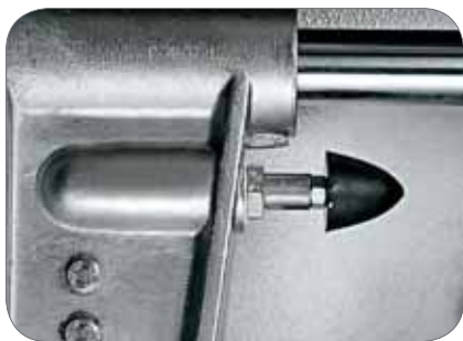
11. Paracolpo carrello Hopper's buffer
